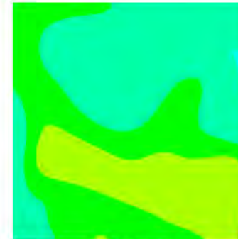
ESP N3 Inlet Average Sorbent Mass Fraction = 3.9 \times 10^{-5} Sorbent Mass Fraction RMS = 10.6%
