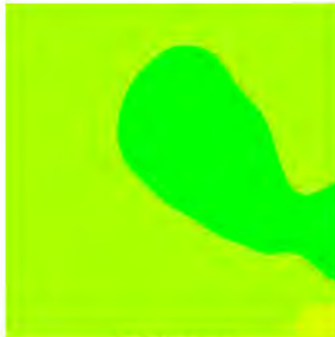
ESP N1 Inlet Average Sorbent Mass Fraction = 4.4 \times 10^{-5} Sorbent Mass Fraction RMS = 3.6%
